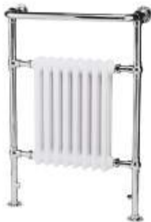
TWW €529 Cashel Traditional Towel Warmer Chrome & White H: 963mm W: 675mm Output: 3520 BTU/hr Pipe Centre: 460mm Watts: 1032
